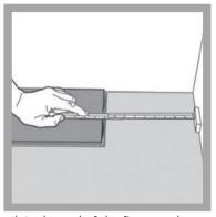
4) At the end of the first row, leave a 1/4" gap, to the wall and measure last plank and cut it off.
