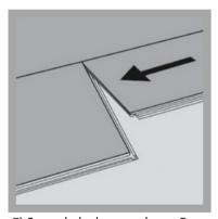
7) Second plank, second row. Drop the plank gently to the narrow end of the previous plank.
