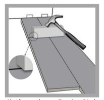
9) Afterwards use Tapping Block and a hammer along both short end joints. Please be careful not to damage the profile or edges during engaging the planks. Test each end joint to make sure it is completely engaged.
