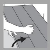
Disassemble the panels by lifting the planks of the row upwards and disengage lock then slide the short ends horizontally apart.
