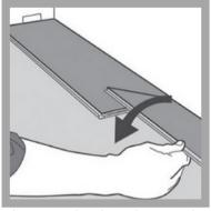
3) During the drop down, make sure the planks are tight against each other. Gently press or tap at the narrow end just installed. (see step 9)
