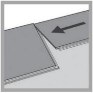
2) Second plank, first row. Drop this plank gently to the narrow end of the first plank.
