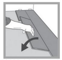
8) Click the plank to the narrow end of the previous plank. During the fold down, make sure the planks are tight against each other.
