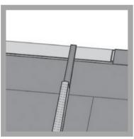
10) Last row. Minimum width 2". Remember to leave a 1/4" expansion gap. Cut the planks lengthwise and glue the short ends.
